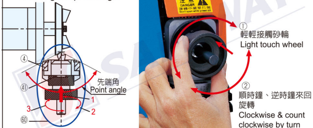
D. 如何研磨鑽頭逃隙角 How to grind drill chisel edge angle
