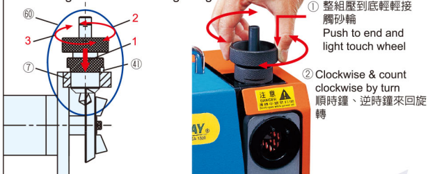
E. 如何更換鑽石砂輪 How to change grinding wheel
