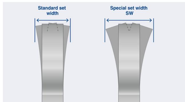
Standard set width compared to special set width SW: The extra wide set increases the free cut of the band saw blade so that there is more clearance to prevent jamming due to released material residual stress.
