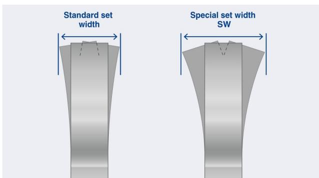
Special set width SW: The extra wide set achieves the free cut of the band saw blade so that there is more clearance to prevent jamming due to decreasing material residual stress.
