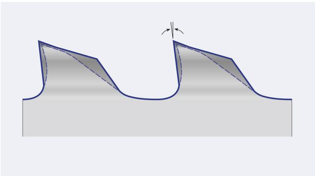
The PROFLEX<sup>®</sup> PREMIUM M42 is equipped with a special profile tooth form, which have a positive rake angle and a reinforced tooth back. The susceptibility
