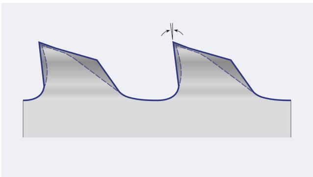
The special profile tooth features a positive cutting angle and reinforced tooth back edge. This reduces susceptibility to tooth breakage and vibration when sawing profiles.
