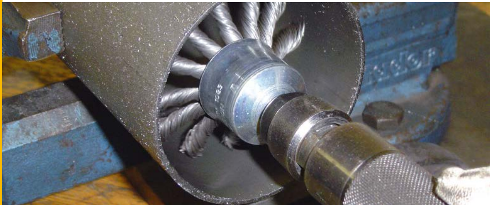
Opening of the end brushes depending on the RPM
